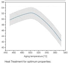
Solution Annealing: 1000°C / 1h soaking time / air cooling to room temperature Ageing: 500°C / 3h soaking time / air cooling
